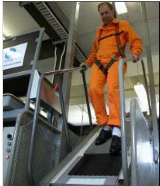
Figure 2: The Ramp Tester uses human subjects to assess the slip resistance of surfaces under controlled conditions
