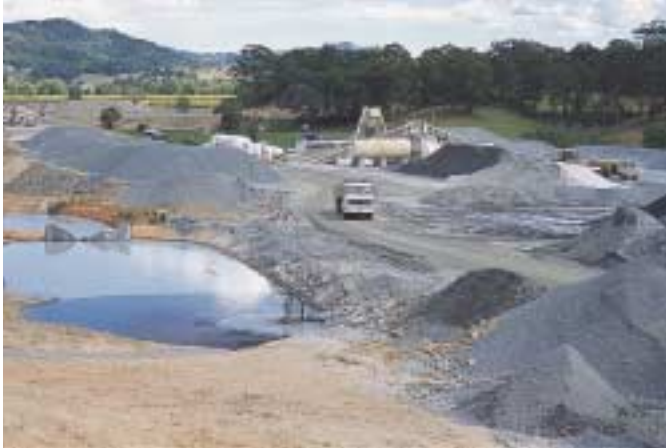
Figure 11: Stockpiling manufactured materials
