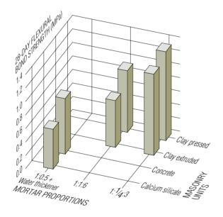
**Figure 2:** Mix and masonry unit effect on 28-day flexural bond strength
