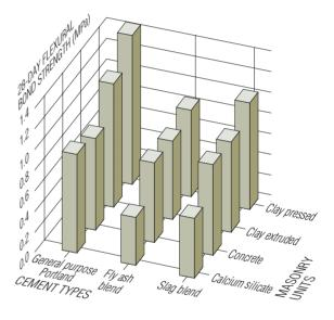
Figure 4: Cement and masonry unit effect on 28-day flexural bond strength
