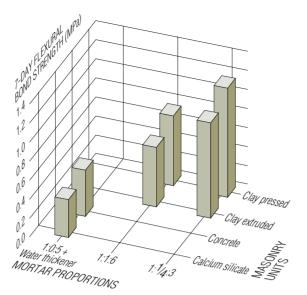
**Figure 1:** Mix and masonry unit effect on 7-day flexural bond strength
