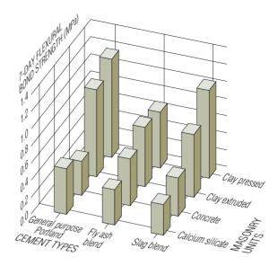
Figure 3: Cement and masonry unit effect on 7-day flexural bond strength
