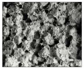
**Figure 6:** Electron micrograph of mortar overdosed with air entrainer
