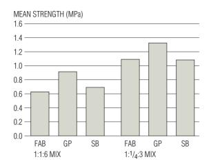
**Figure 5:** Mortar mix and cement effects at 7 days age for clay bricks
