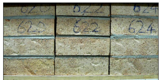
Raked finish Ironed finish Flush finish Three finishes used in the study
