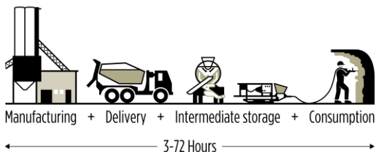
Figure 5.14 – HCA Used to Extend Working Time
