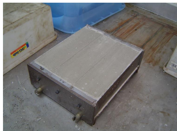
Figure 26.13 – Three Drying Shrinkage Specimens Cast in a Mould
