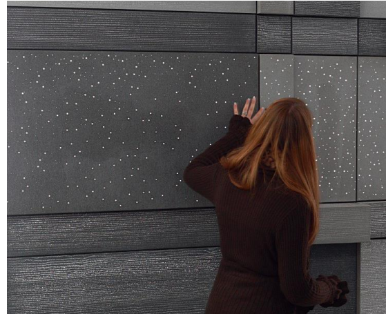
Figure 24.4 – Translucent Concrete Booth at Expo Bau 2011 in Munich, Germany 24.4
