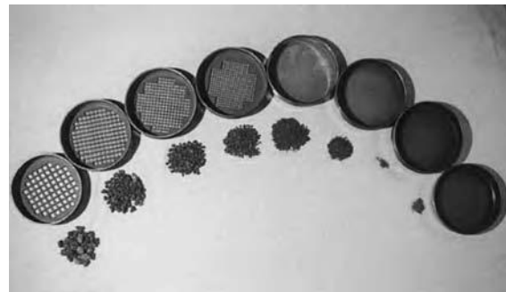
Figure 25.3 – Aggregate Combined Grading determined by Sieving
