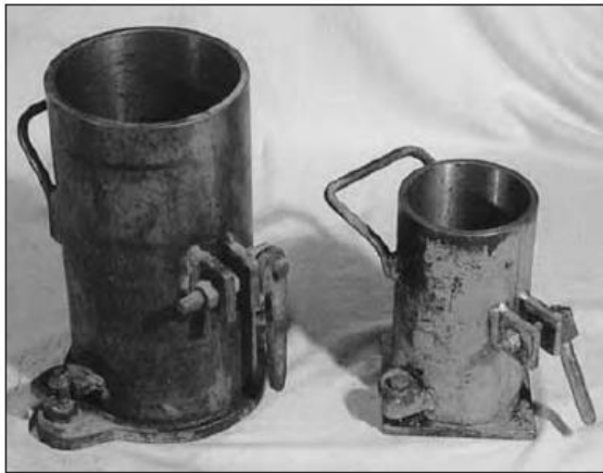
Figure 26.8 – Moulds for the Two Standard Sizes of Concrete Test Cylinders
