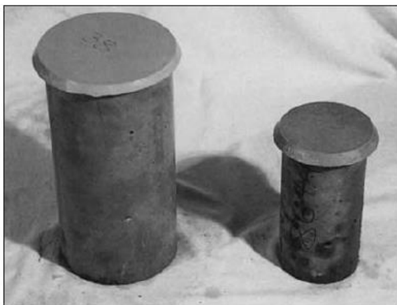
Figure 26.9 – Sulphur Capped Concrete Test Cylinders in the Two Standards Sizes
