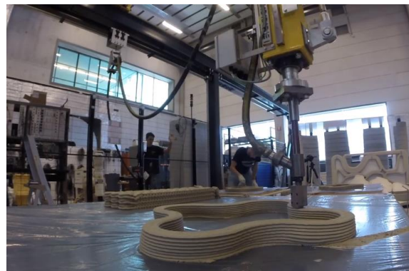
Figure 24.7 – Robotics and 3-D Printing, Extrusion-based Technique 24.7
