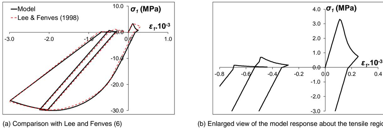
**Figure 2. Numerical results of loading with multi-cycles: (a) Comparison with Lee and Fenves (6), (b) Enlarged view of the tensile region in (a).**
