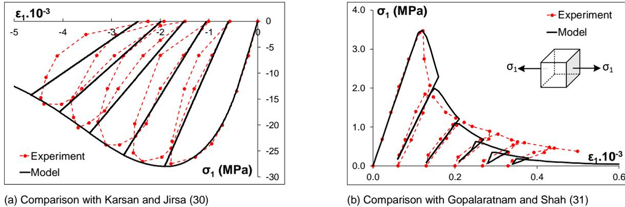
**Figure 1. Comparison of cyclic behaviour of concrete: (a) compression-only, (b) tension-only**
