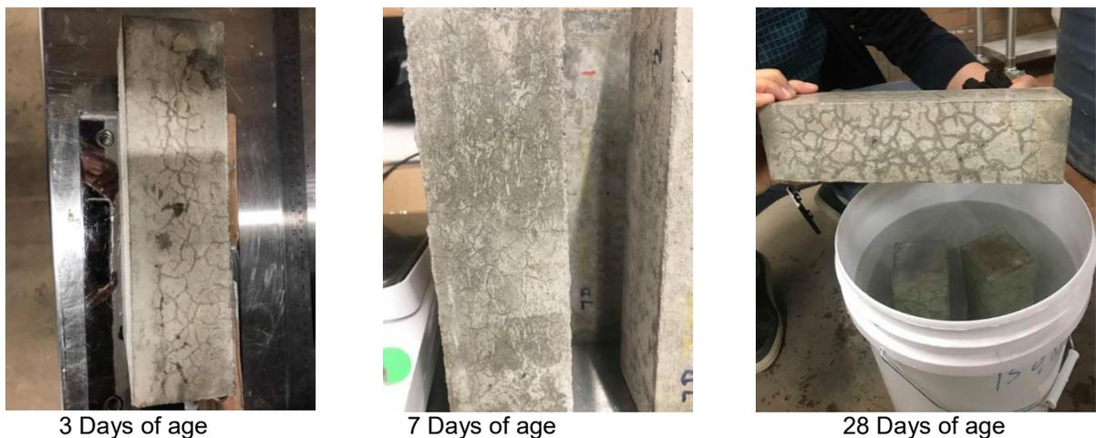
**Figure 5. Crack patterns of reactive aggregate B prisms with 3%  $\text{Na}_2\text{O}_{\text{eq}}$  boosting after 3 cycles of autoclaving at ages of 3, 7 and 28 days**
