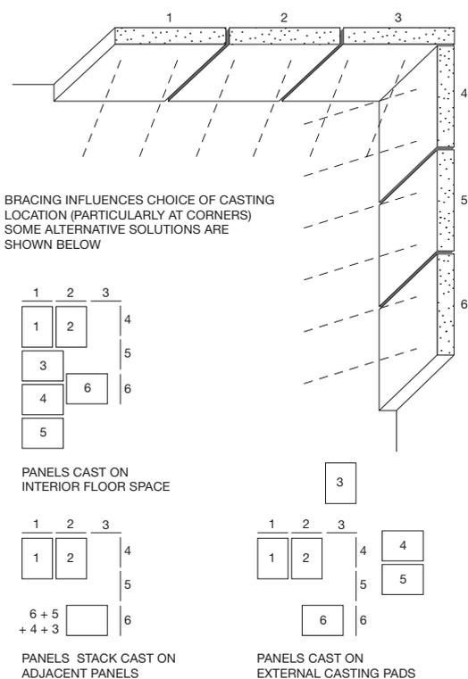
Figure 10.2 Influence of Bracing on Casting Layout
