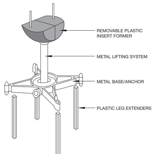
Figure 10.5 Typical Face-Lifting Insert
