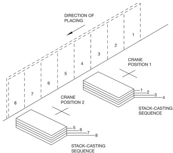
Figure 10.1 Stack-Casting Sequence
