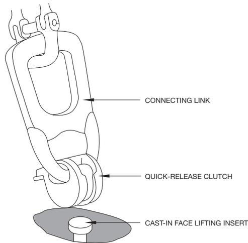
Figure 10.6 Typical Quick-Release Lifting Clutch
