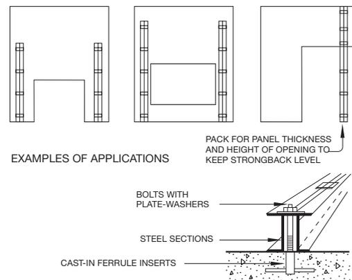
Figure 10.10 Use of Strongbacks to Strengthen Panels During Erection
