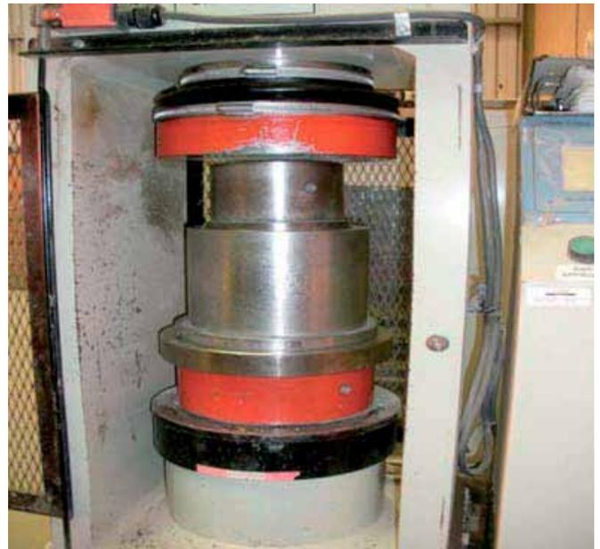
**Figure 7: A Wet/Dry sample under test in a compression machine**
