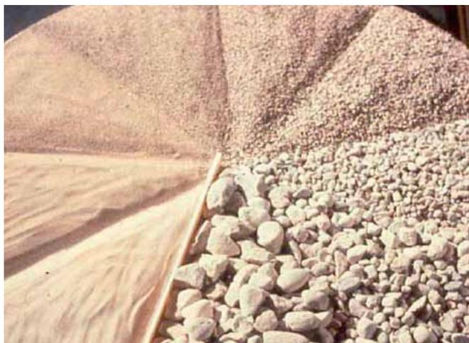
Figure 2: A sample graded into its individual sizes
