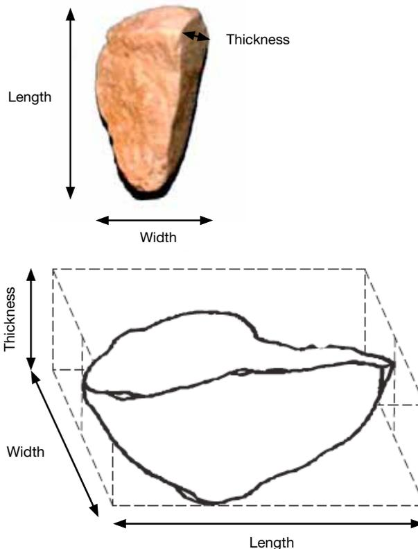
Figure 3: Standard stone dimensions
