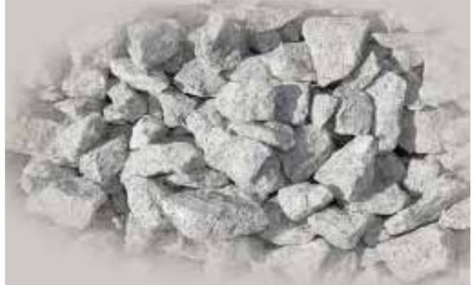
Figure 8: A sample of typical Gabion or Mattress rock.
