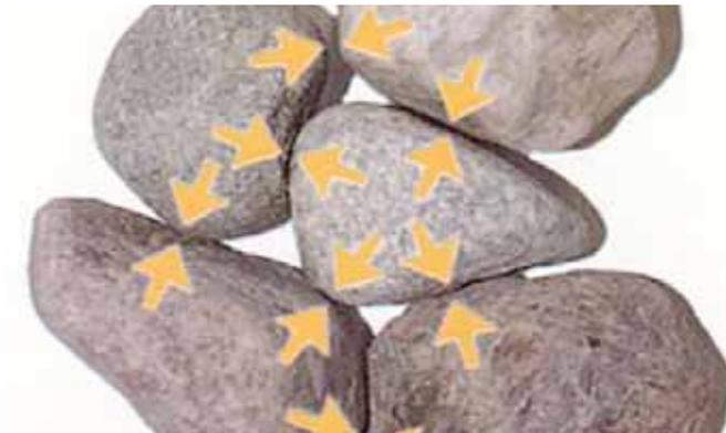
**Figure 7: Diagram showing rock- on-rock contact and transfer of load at these points**
