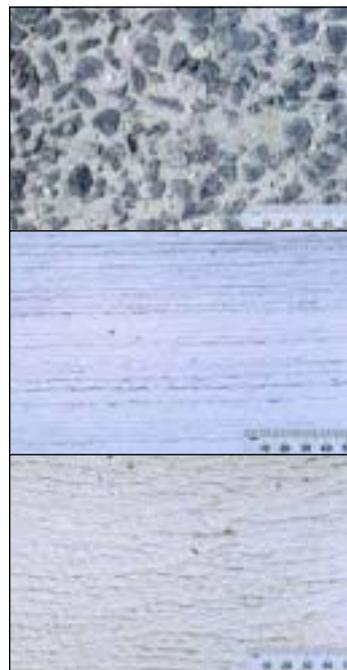
**Figure 5:** The exposed aggregate (top), broomed (middle) and wood floated (bottom) finishes, shown with a 50 mm scale.
