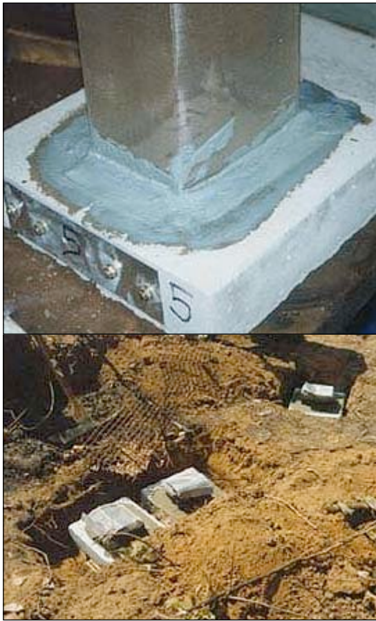
Figure 1: Test slab preparation and placement into position at exposure sites
