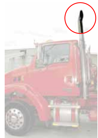
Figure 2 Exhaust vented above cabin height
