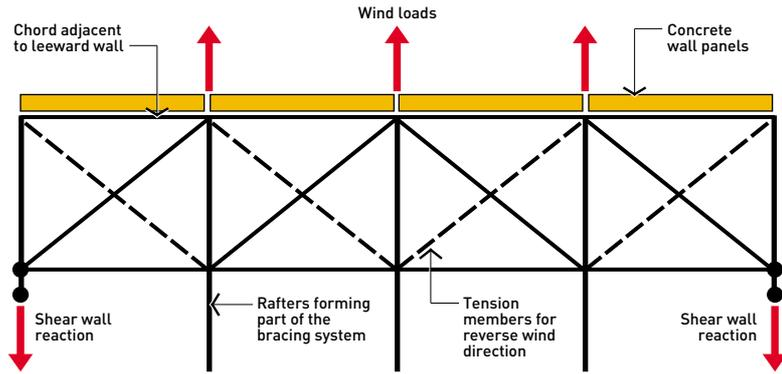
**Figure 8: Alternate model for wind truss analysis**
