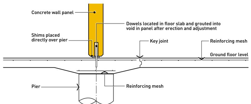
**Figure 30: Typical connection of suspended floors**
