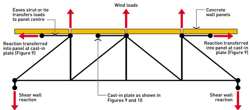
**Figure 9: Transfer of loads into panel**
