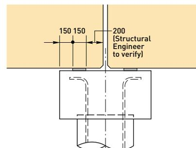
**Figure 25: Use of timber piles with pile caps**
