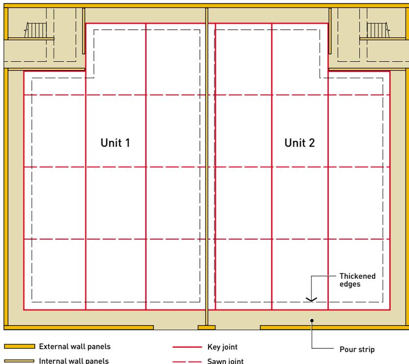
panels to allow the completion of the floor slab once the panels have been erected, **Figure 29 (a)**.
