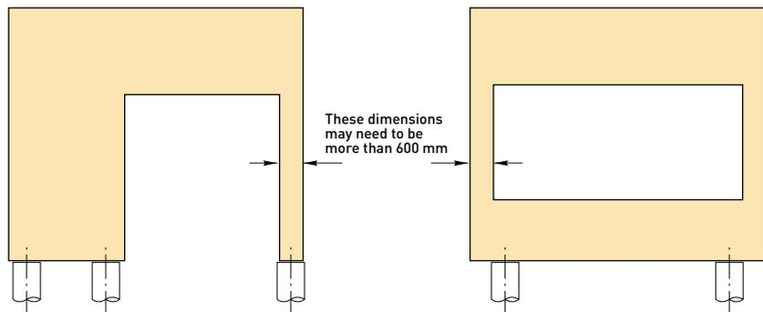
**Figure 4: Situations where leg or mullion widths could be less than 600 mm**
