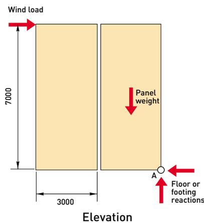
Referring to **Figure 18**, if two larger panels (of typical precast width) of similar dimensions are used (ie total 6000 mm wide, 7000 mm high and 150 mm thick) the capacity is as follows:
