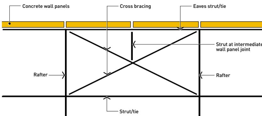
Figure 13: Strut to support joint at smaller panel
