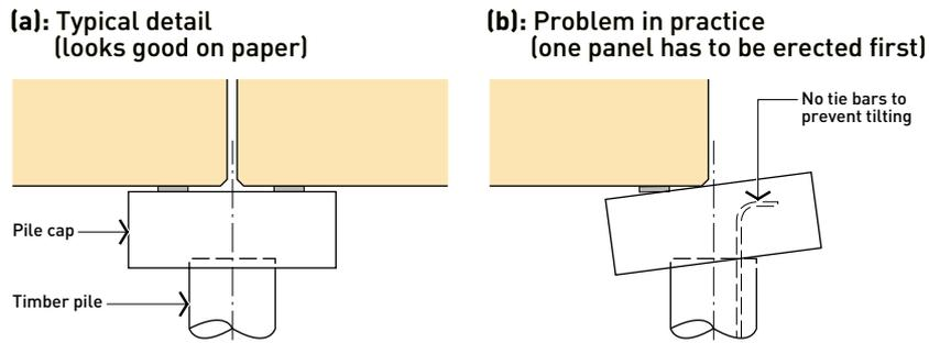
The starter bars, which connect the pier or pile and the capping member, do their work (resisting eccentric loads) while the panels are being erected. Note that with the use of timber piles, no starter bars are provided. With both panels resting on the pile cap, the load on the pile is balanced and there are no problems. However, if one panel has to be erected first, it will cause an eccentric load and possible movement of the pile cap, **Figure 25**.
