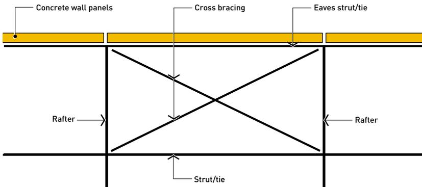
Figure 12 : Strut to support joint between smaller panels
