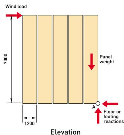
**Figure 18: Two larger panels as shear wall**
