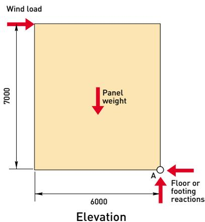
or twice that of two smaller panels. Thus it is particularly important to check stability under shear loads when using narrow panels in lieu of wide elements.
