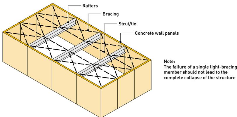
**Figure 6: Brace each bay to transfer lateral loads on the walls to the supporting cross walls**
