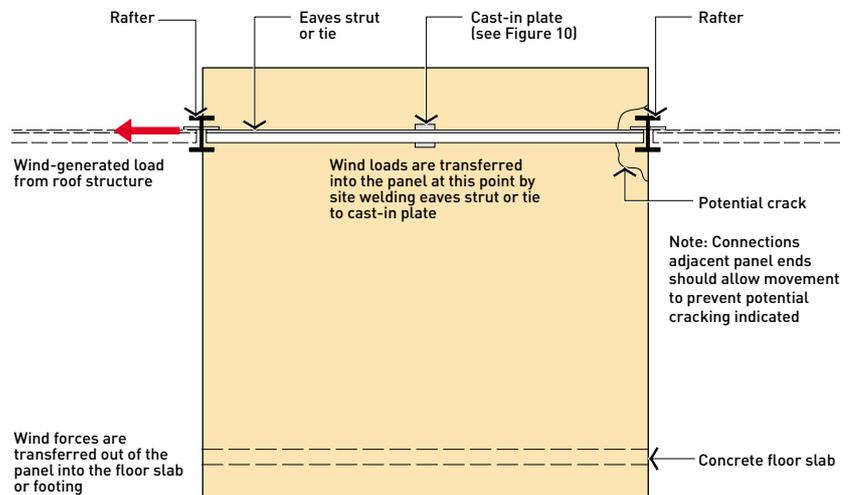
**Figure 10: Eaves strut or tie welded to cast-in plate**
