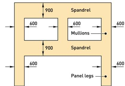
**Figure 3: Situations where leg or mullion widths may need to be more than 600 mm**
