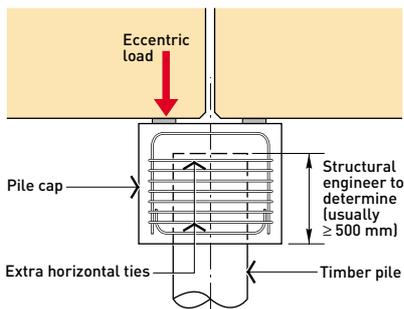
**Figure 27: Pier/pile and cap levels**
