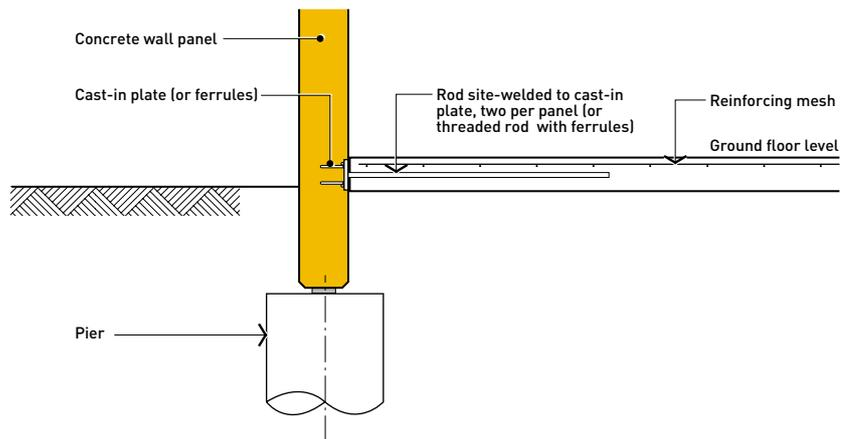
**(c): Internal wall panel, supported on floor slab**
